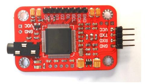
Once the group is important, it will output message through serial port. It could have 15 voice instructions in 3 groups. Each time you need to import the group before it could recognize instructions in that group. That means, this module could recognize 5 voice instructions at the same time. In recognition stage, this module could receive other serial commands. It will not exit the recognition stage until you send **0xAA00**, or delete that group, or begin recording instructions.
